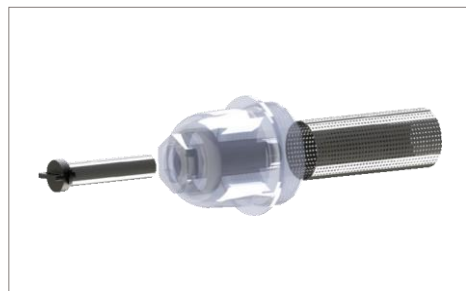
Remove magnet by turning 90° then clean mesh and glass from any debris. Check conditions of O-rings and seals
