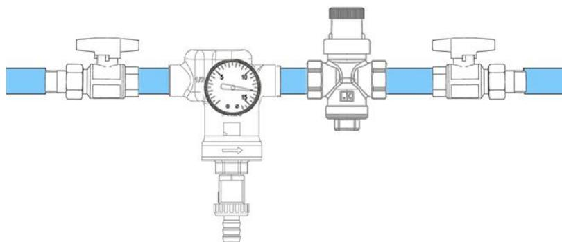
When there is a device which produce or store hot water or pipes are exposed to sudden changes in temperature, an increase of outlet pressure may occur; this event is due to the raise in pressure that follows the temperature rising: an expansion vessel between downstream the pressure reducing valve will avoid this problem.
