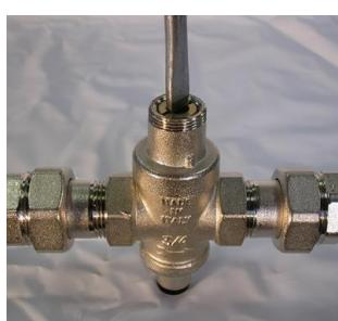
All Malgorani pressure reducers are tested before being packaged; during the test they are set at the outlet pressure of 3 bars; outlet pressure can be easily adjusted once the pressure reducing valve is installed on site.
