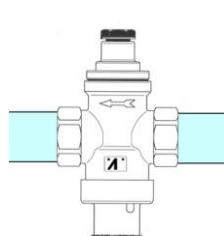
The pressure reducers MINIBRASS don't get the effects, in their functioning, of gravity force; therefore they can be installed in the plant in any position:
